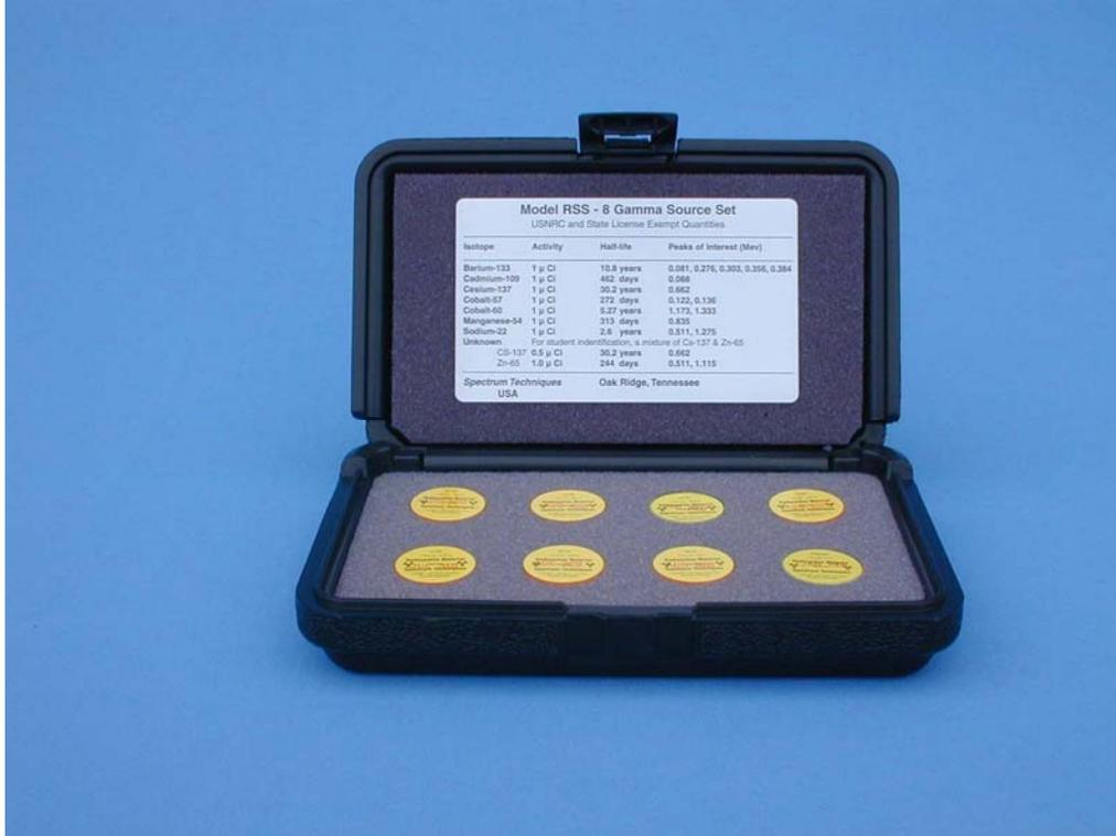
Figure 3: Kit of eight different gamma sources.
