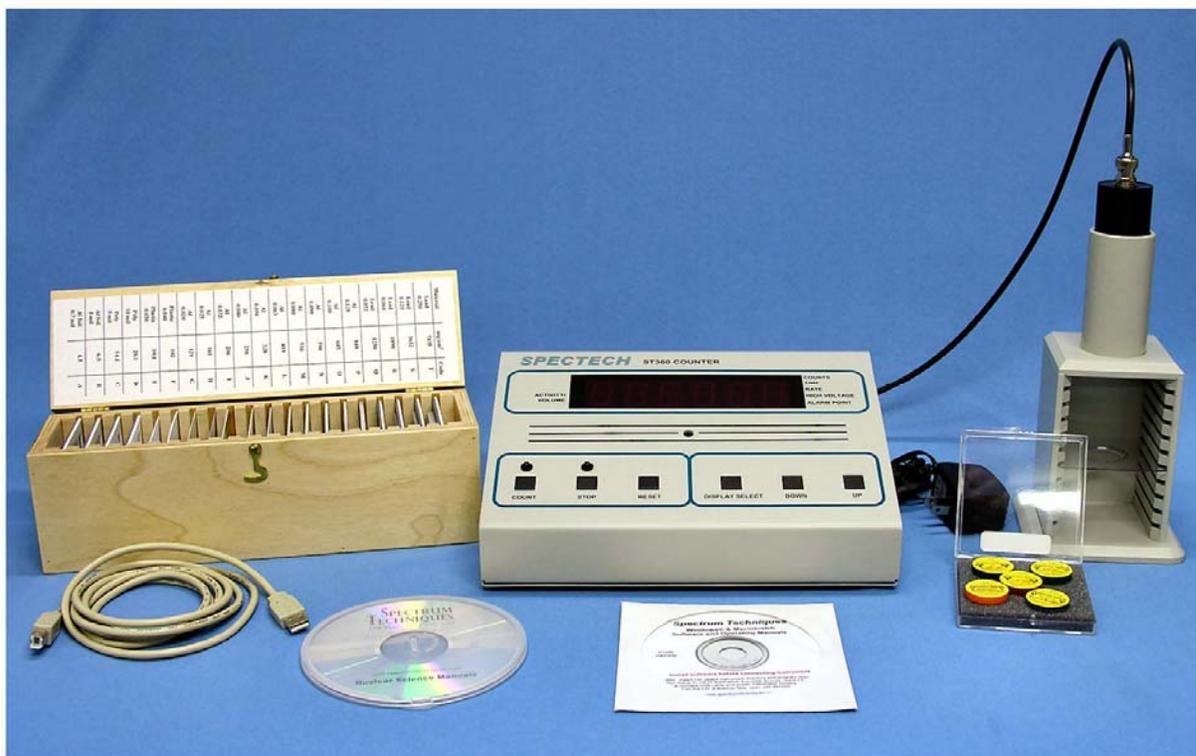
Figure 2: Setup for ST360 with sources and absorber kit.
