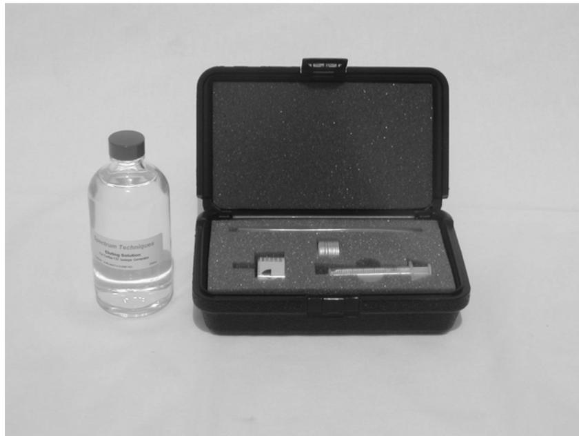
Figure 3: Isotope Generator to make Ba-137m from Cs-137
