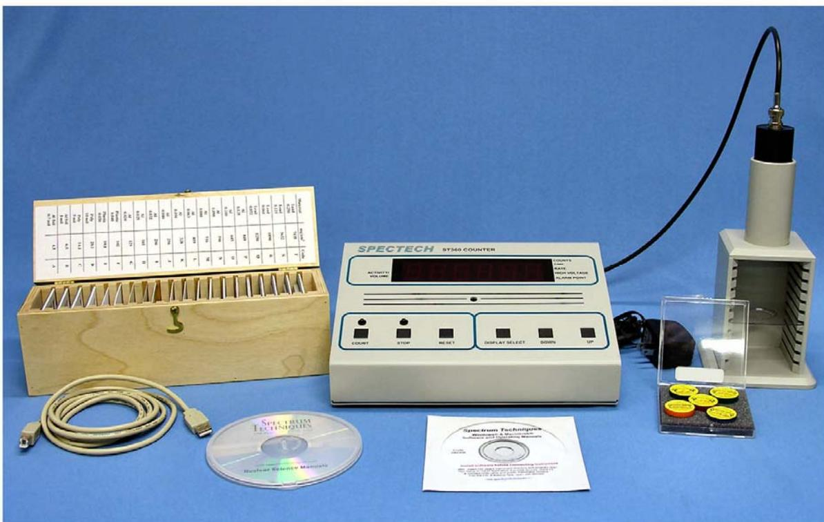
Figure 2: ST360 setup with sources and absorber kit.
