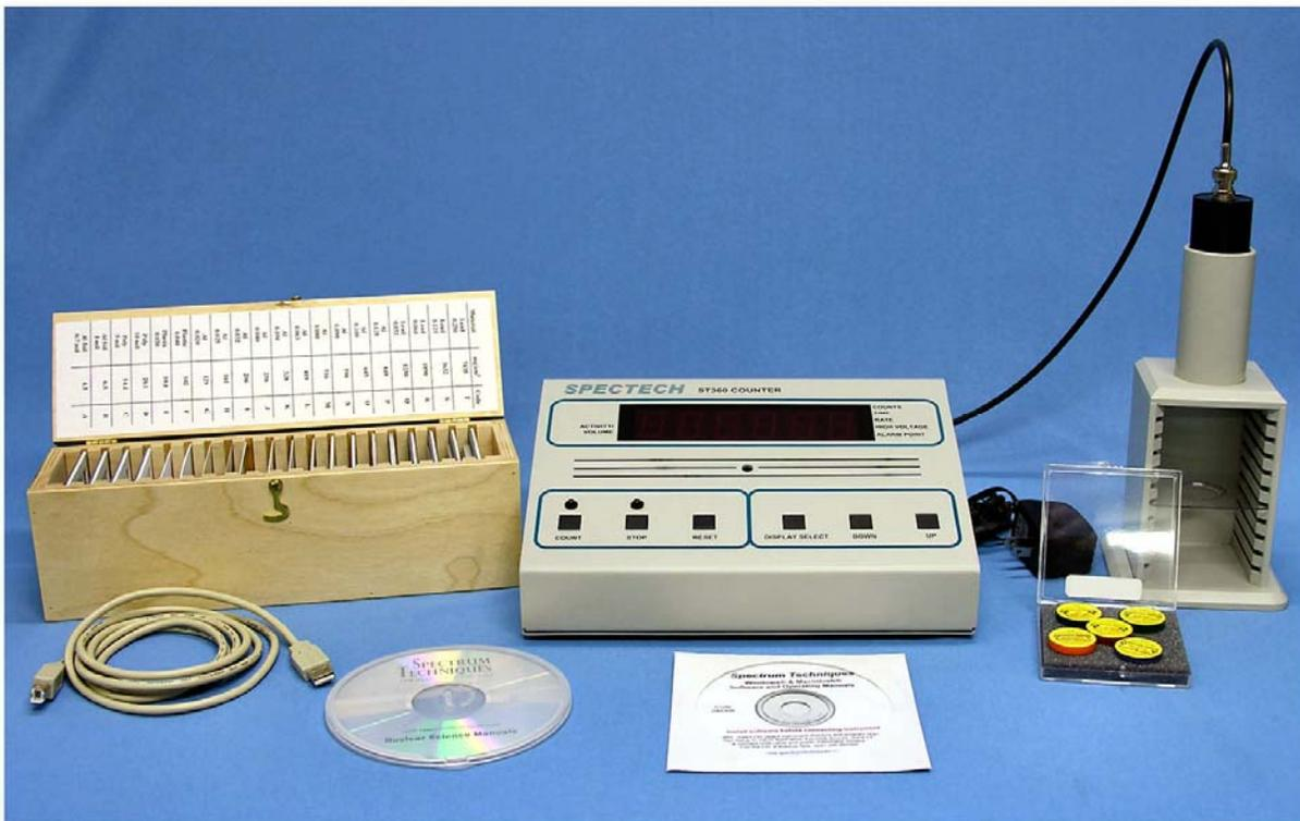
Figure 1: Setup for ST360 with sources and absorber kit
