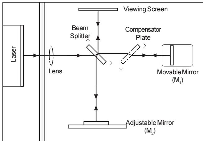
Figure 1. Michelson Interferometer
