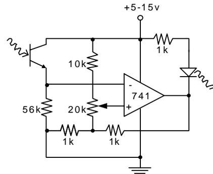
The phototransistor should be mounted in a plate of sheet steel, which can then be held in the magnetic viewscreen holder. Mask the transistor with a piece of electrical tape with a pinhole at the center. Adjust the sensitivity of the circuit with the 20k potentiometer so that the flashes of the LED can be counted instead of the actual fringes.
