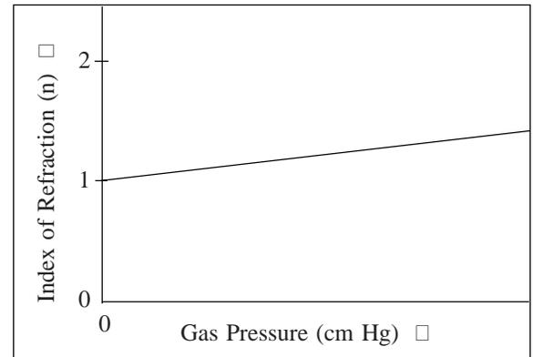
Figure 2.1. Index of Refraction versus Gas Pressure
