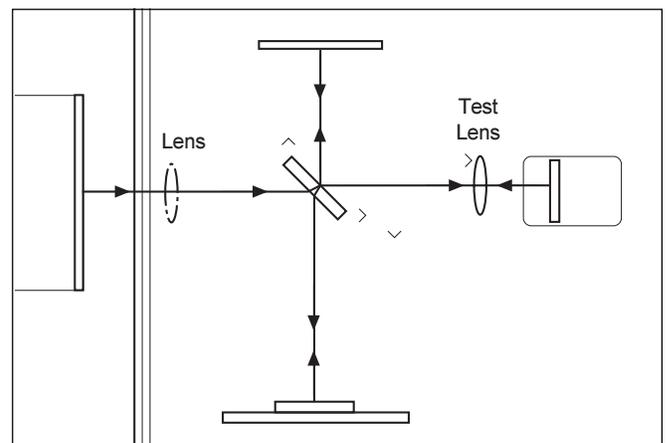
Figure 3. Twyman-Green Interferometer
