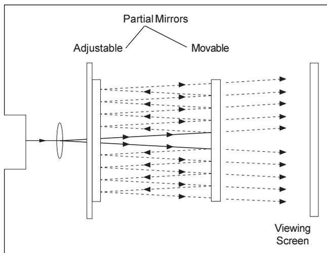
Figure 4. Fabry-Perot Interferometer
