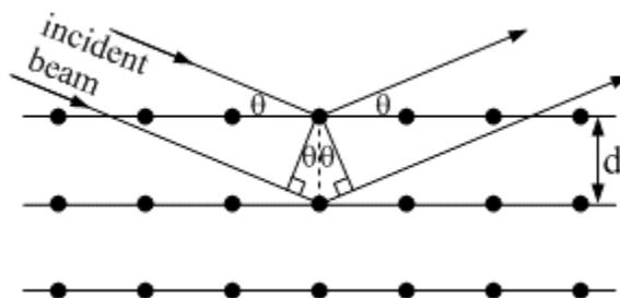
**Figure 2. Electron Waves Reflected from Atomic Planes.**
