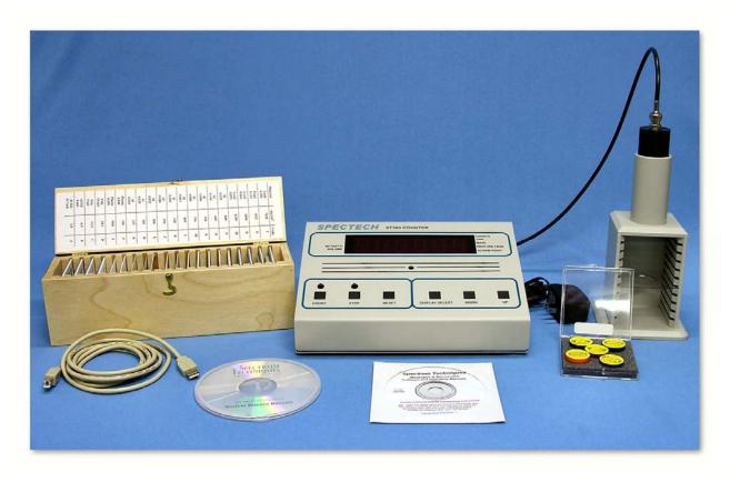
Figure 2: Setup for ST360 with sources and absorber kit.
