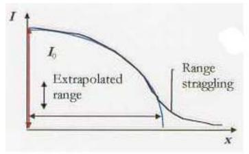
Figure 1: Typical absorption curve for beta particles. Plot is of intensity (activity) vs. absorber thickness (x)
