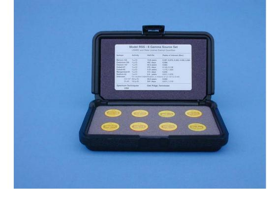
Figure 3: Kit of eight different gamma sources.
